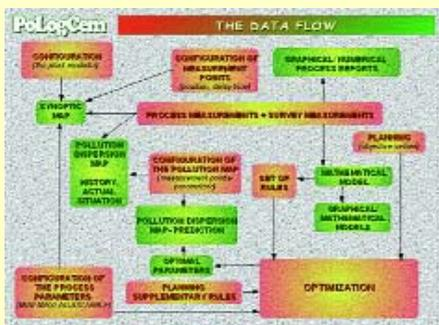
Figure 1. Data flow in the PoLogCem software
