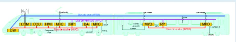
Figure 2. Electronic control and supervision system for a train unit
